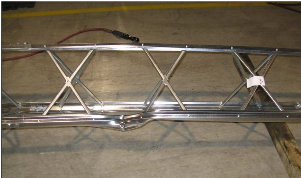
Figure 2: Failure of DMX-68N tower
